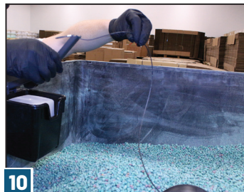
10 While holding the activation arm in the upward position, place the anchor weight on top of the seed in the center of the box.
