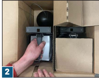
2 Lift the activation arm securely and pull the cardboard arm support towards the side of the box.
